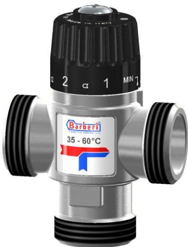
Barberi L-Comfort Series thermostatic mixing valves are devices with mixed water on the side way and are used to regulate the water temperature. They are used in sanitary water plants, heating circuits, in heating plant, in heat generators (hang-wall boilers, wood boilers, heating pumps) and industrial water plants. Their purpose is to maintain constant the mixed water temperature of the utility even when temperature and inlet pressure could vary at the hot and cold water inlets.
