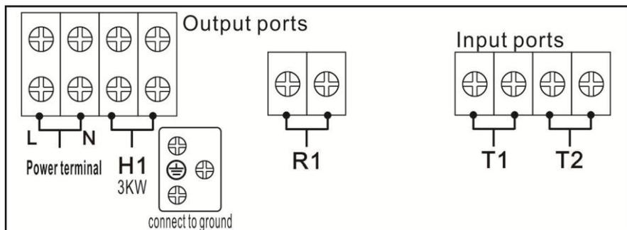
➤ **Power terminal N, L:** AC220V, 20A, for power connection, L: live wire, N: zero wire,  $\oplus$  protective wire, please connect to ground reliably.
