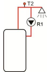
Startup condition for temperature controlled mode (STAT): when tank temperature T1 is 2°C higher than the preset switch-off temperature(CYCF), and then DHW circuit pump is triggered.
