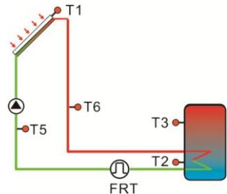
**i** **Note:** when rotary vane flow meter (FRT) is selected for thermal quantity calculation, then it needs to activate FRT (FRT ON) under menu FS/FRT.
