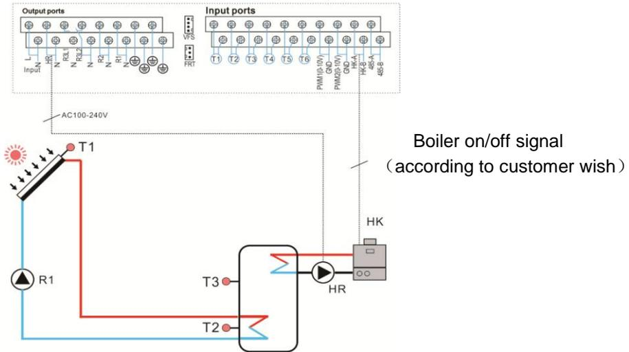
When boiler as back-up device is selected, then back-up heating (HK and HR) is controlled by tank's sensor T3 or T2 (selectable), if the T3's or T2's value is lower than the switch-on temperature of back-up heating, the output relay HK and HR is switched on, when T3 or T2 is higher than the switch-off temperature of back-up heating, the output relay HK and HR are switched-off.
