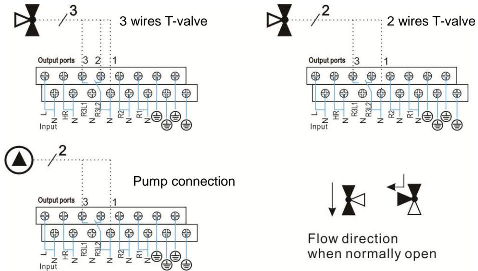
When R3 is for controlling 3 ways electromagnetic valve, (3 is normally open port, 2 is normally close port, 1 is common port)
