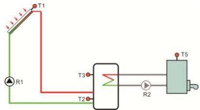
1. The temperature difference between the sensors of heat source T5 and heat sink (T3 as priority selection) has exceeded the switch-on temperature difference.
