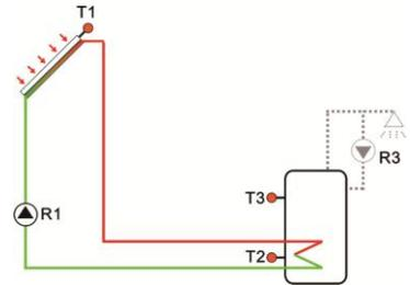
● **Temperature controlled DHW pump within the preset 3 time sections**
