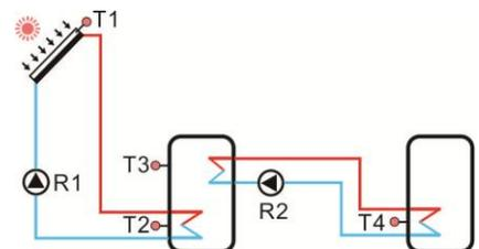
3. Temperature of object tank is lower than its preset maximum temperature.
