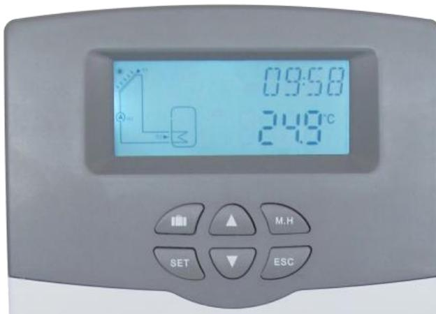
➤ Controller is operated with the 6 buttons on the right side of the screen
